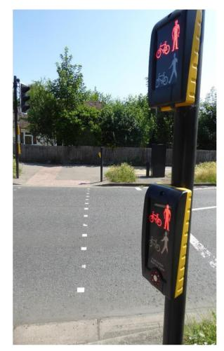
Toucan crossings are designed for both pedestrians and cyclists and are typically used adjacent to a cycle-path. Cyclists should dismount to cross the road using Zebra, Pelican or Puffin crossings.
